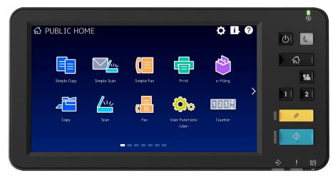
Access the systems functionalities via an intuitively operable 26 cm (10.1") tablet-style touch screen. It is equipped with an embedded web browser and is fully customisable, allowing you to tailor settings and automate workflows – including integration of third-party solutions. In line with the new look and feel of the e-STUDIO series, the bold and straightforward user interface, enables simple operation and improved efficiency.
