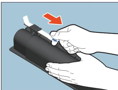
6 Align the new toner cartridge to the guide. Insert it up to the black line.
