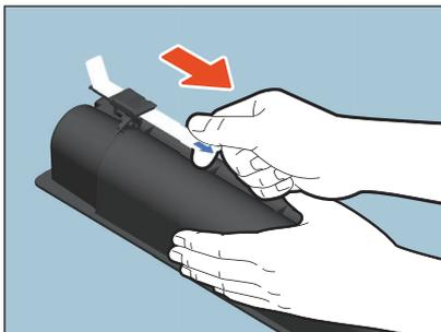
**6** Align the new toner cartridge to the guide. Insert it up to the black line.
