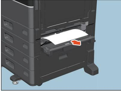
If the paper is misfed on the cover side, remove it as shown in the figure below.
