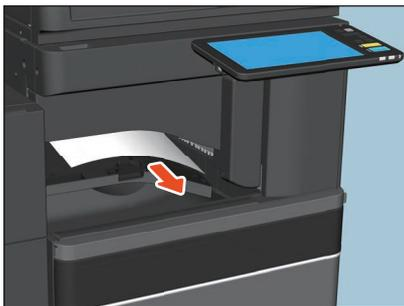
**7 If the paper size is small, turn the knob shown in the following figures to send the paper, and then remove the misfed paper.**
