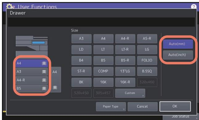
Press [User Functions -User-] on the Home screen > [Drawer] and select the desired drawer on the displayed screen. Select [Auto (mm)] when A/B format paper is loaded and [Auto (inch)] when LT format paper is loaded. The paper sizes for all drawers are preset to [Auto (mm)] or [Auto (inch)] depending on your region. If you do not need to change the setting, you do not need to do this procedure.
